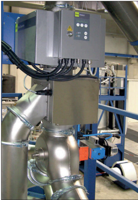
Installation example: Metal separator RAPID VARIO-FS used for the quality control of PET regenerate. (old version)
