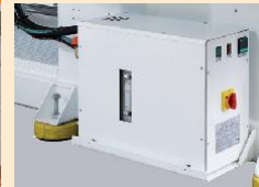
CLOSED CIRCUIT CENTRAL UNIT TO COOL MOTORS, ROLLER SCREWS AND BEARINGS. MOTORLAR VE RULOLU VİDALAR İÇİN KAPALI DEVRE SOĞUTMA ÜNİTESİ
